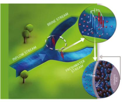
Porous carbon electrodes can be used to desailnate water
