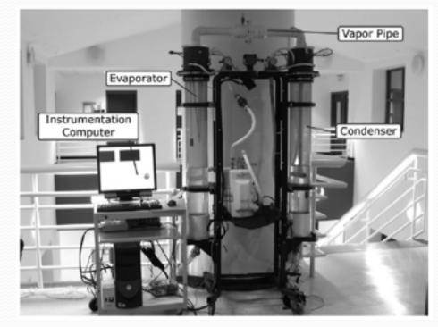
Fourth floor portion of the proof of concept. Hoses extend down 10 m to reservoirs on the 2<sup>nd</sup> floor. From B.A. Moore et al/ Desalination 220 (2008) 502-505
