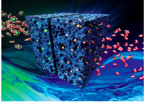
Flow-through electrode capacitive desalination uses a new hierarchical porous carbon material to create a new device geometry in which the feed stream passes directly through the electrodes, resulting in significant improvements to salt removal and desalination rate.
