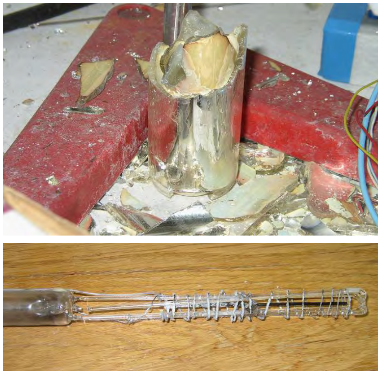
Figure 12.2. The remains of a cell that exploded in September 2004, Université d'Aix-Marseille II. Photo courtesy J-P. Biberian.
