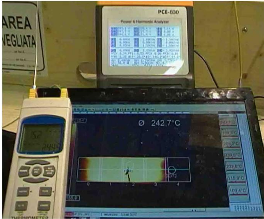
Fig. 13. Dummy measurement set-up. Center: laptop display showing the thermal image of the dummy divided into 5 areas, and the dark shadow of the thermocouple, with probe point located under a dot. Left: thermocouple LCD display, indicating a temperature of 244.5 °C. This is relevant to the same area which the IR camera reading of 242.7 °C, visible on the laptop display, refers to. Lower thermal exchange between the probe and the environment is the most likely cause for the difference.
