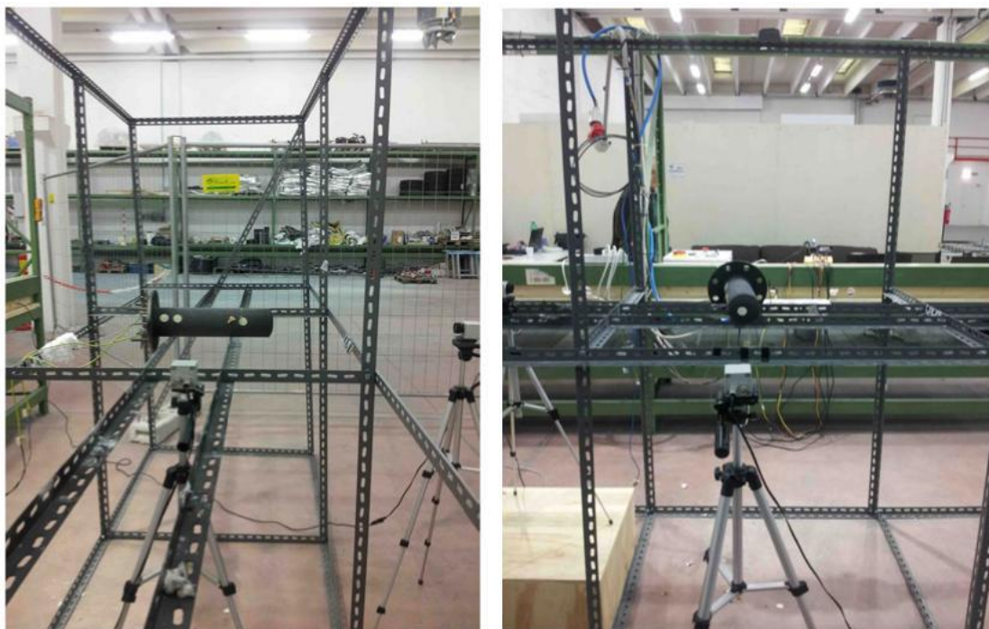
Fig. 12. Two images of the E-Cat HT2. The first displays one of the sides, as framed by one thermal camera, the second displays the “top”, framed by the second IR camera. The adhesive “dots” used to evaluate paint emissivity are visible in both images. Note how, in the image on the left, one of the dots is about to fall off due to the heat from the underlying area.
